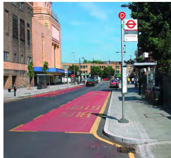
Figure 2.15: Bus Stop Protected by a 'Bus Cage'
