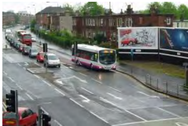
Figure 2.13: Bus Lane with Pre-Signals
